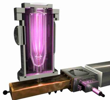
Figure 1: Low-pressure microwave plasma reactor.
