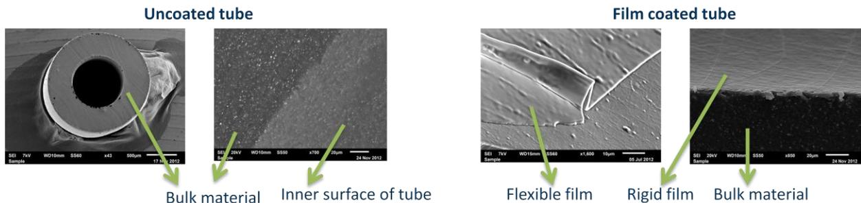
Fig. 2. SEM images of uncoated and film coated plastic tubes (catheters).
