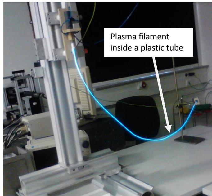
Fig. 1. Filamentary plasma ignited inside a plastic tube (catheter) in argon precursor mixture in order to coat film on the inner surface of the catheter (length 150 cm, tube thickness about 50  $\mu\text{m}$ , inner diameter  $< 2$  mm).
